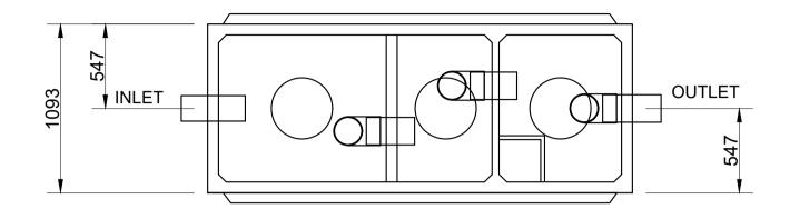
Lid thickness standard at 80mm. Recommended maximum loose soil cover depth - 400mm
